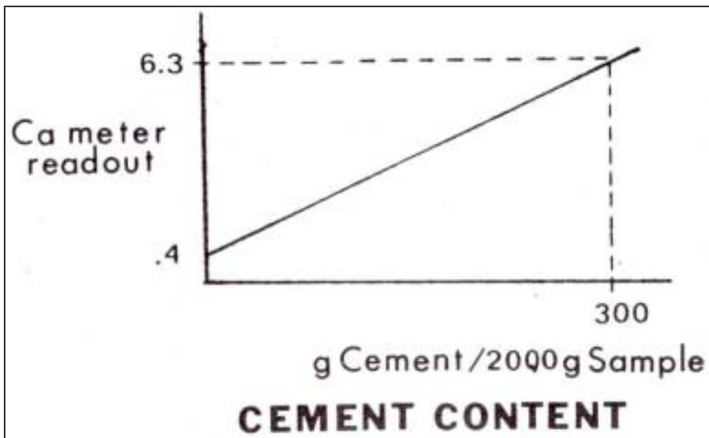
Fig. 5. Calibration Graph for Procedure B
