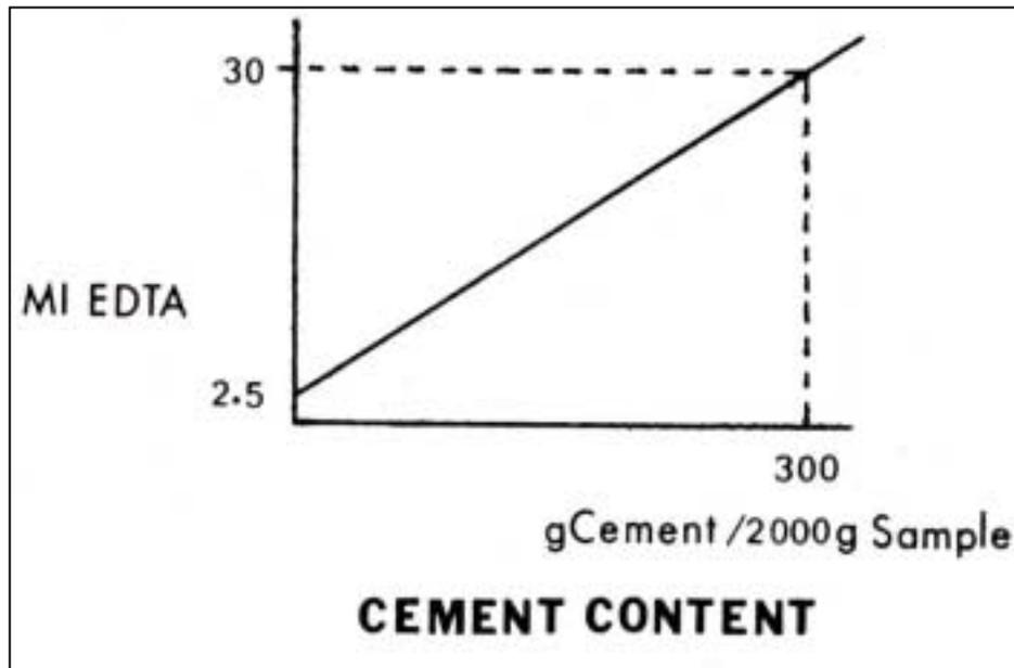
Fig. 3. Calibration Graph for Procedure A
