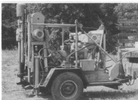
Figure 1. Trailer mounted drill rig
