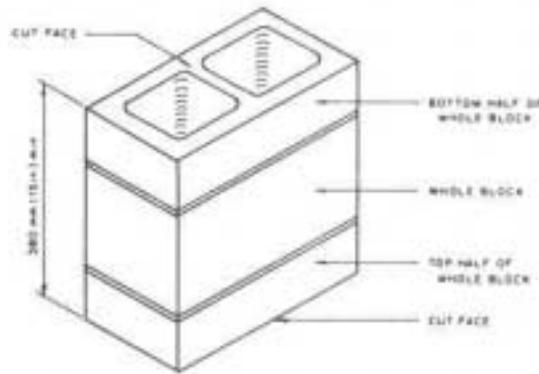
Fig. 1. Masonry Prism Construction for 200-mm (8-in.) High Units
