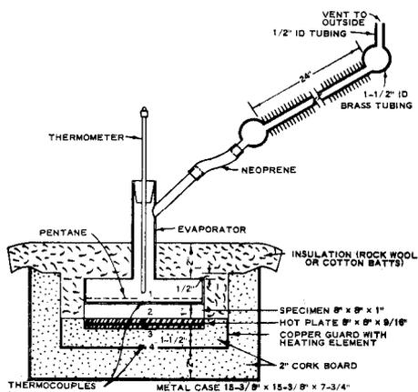
Fig. 1. Thermal conductivity apparatus-general layout
