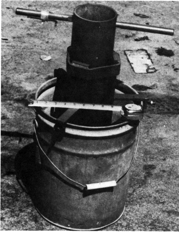
Fig. 1. Prototype tremie flow test apparatus.
