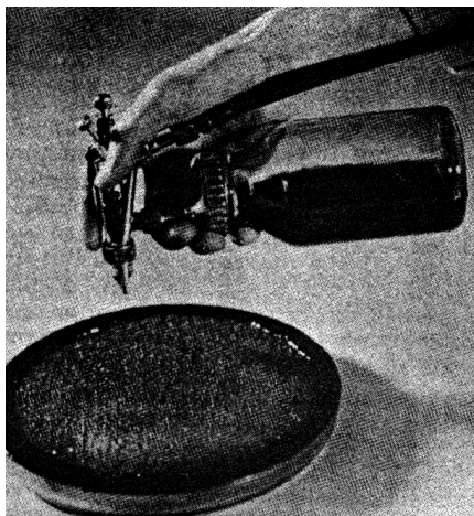
Fig. 2. Applying curing compound to mortar test specimen
