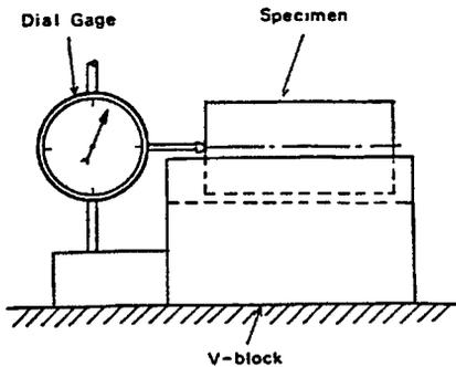
Figure 3. Assembly for Determining the Perpendicularity of End Surfaces to the Specimen Axis
